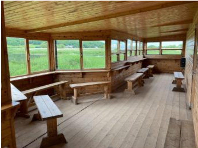
Grisedale Hide showing bay window and low level window for wheelchair users
