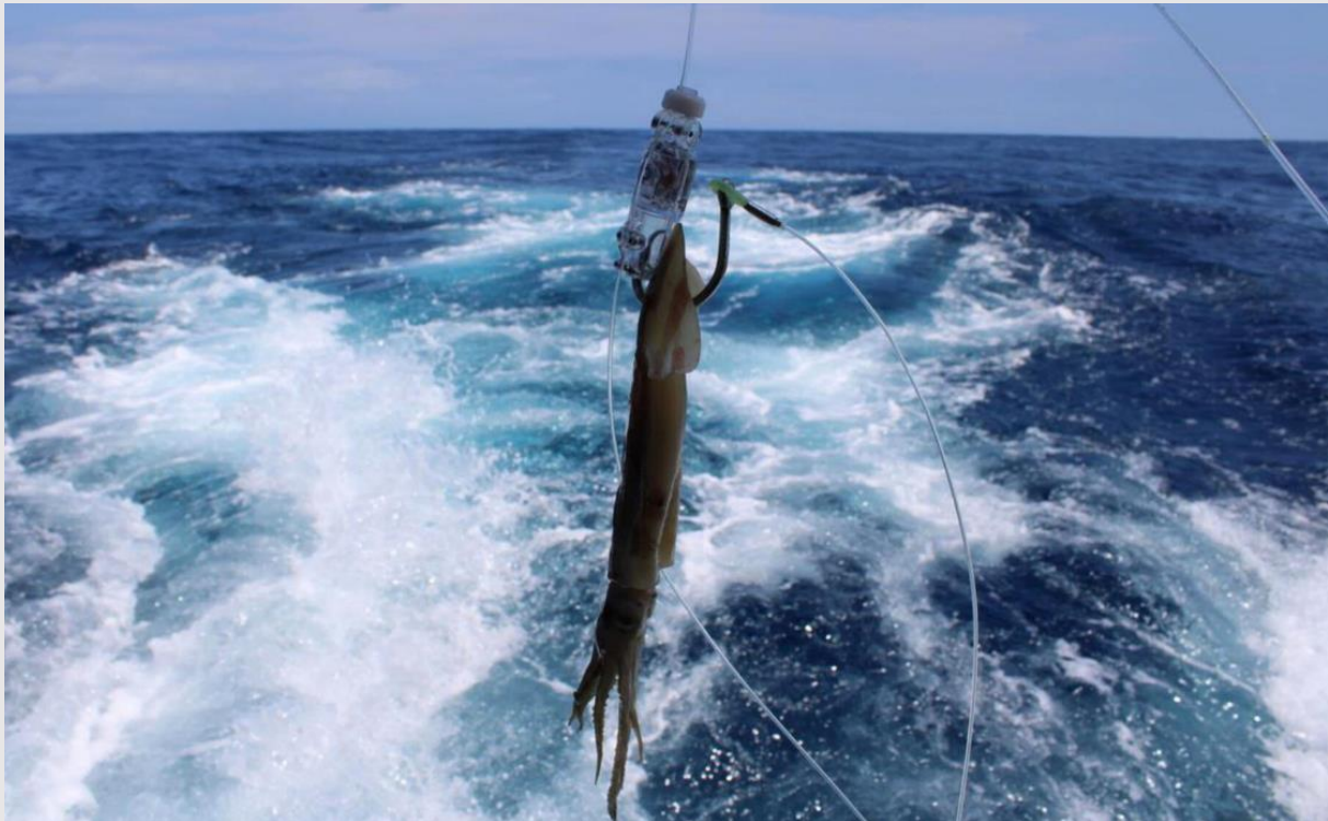
Image: Baited Hookpod ready for deployment, during at-sea trials with the South African pelagic longline fleet.
